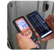
Wireless communication transfer measurement data via Bluetooth, in „live“ mode, to the Sonel Multimeter Mobile application.
