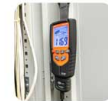
Current logger The integrated current logger with an RTC can be configured with the logging start date and time and up to 24 hours of current logging with a refresh rate of 1 second.
